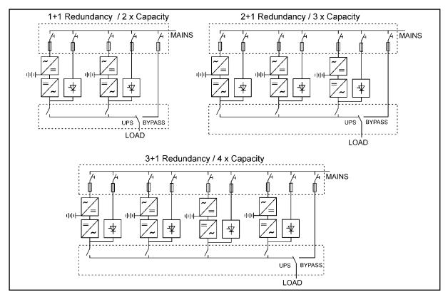
Figure 19 Parallel configurations with UPS modules.
